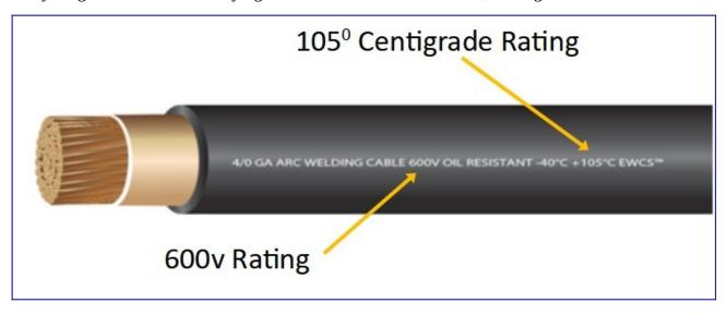
Also, it is important to note that when dealing with DC currents in solar power systems (SPS) you need a high-quality wire with a good insulation rating; 105 degrees centigrade is commonly referred to as the standard. Voltage rating should be at least "600V".
